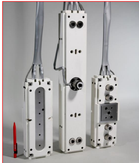
Figure 1 Special enclosures reduce heat losses
